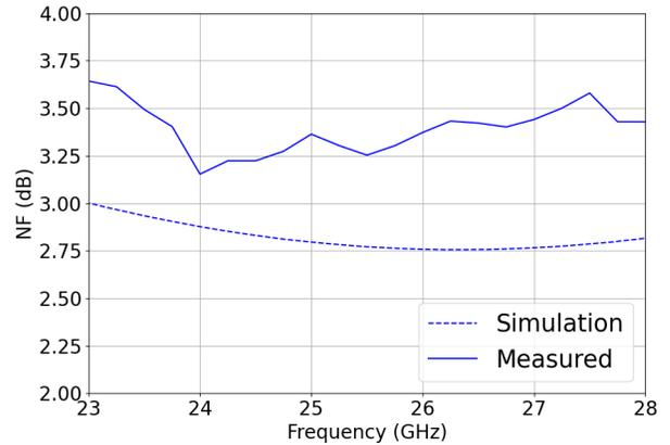
Fig. 5: Simulated and measured NF of the LNA across the frequency band
