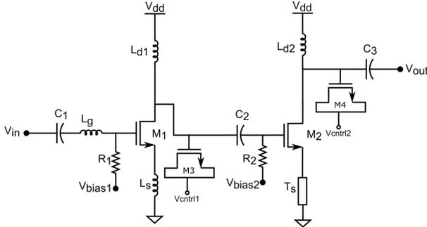
Fig. 1: Schematic view of 26GHz tunable LNA
