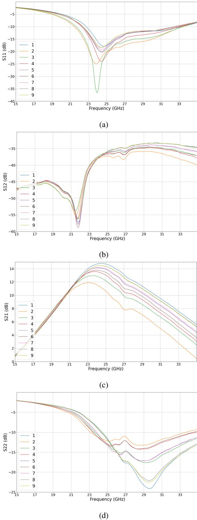
Fig. 4: Measured (a) S11, (b) S12, (c) S21 and (d) S22 of the LNA at different varactor control voltage combinations (refer Table II)
