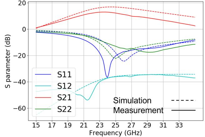
Fig. 3: Measured and simulated S-parameters of the LNA at varactor  $V_{cntrl1}=0.4 \text{ V}$  and  $V_{cntrl2}=0.5 \text{ V}$
