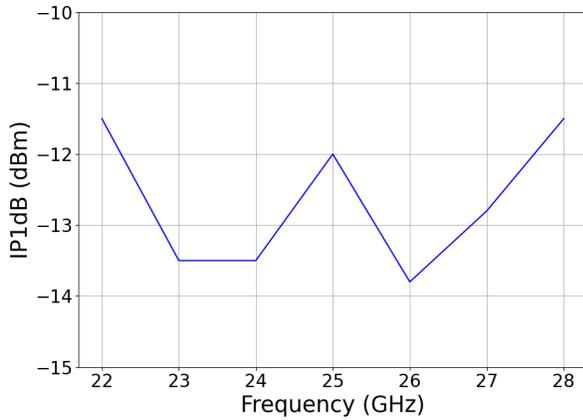
Fig. 7: Measured P1dB points across the frequency band
