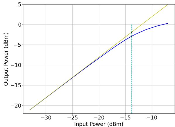
Fig. 6: Measured linearity characteristics of the LNA at 26GHz
