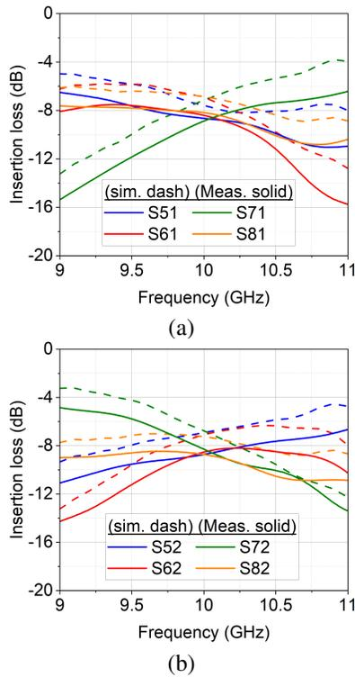
Fig. 4: Magnitude response of the Butler matrix when excited through (a) Port 1 and (b) Port 2
