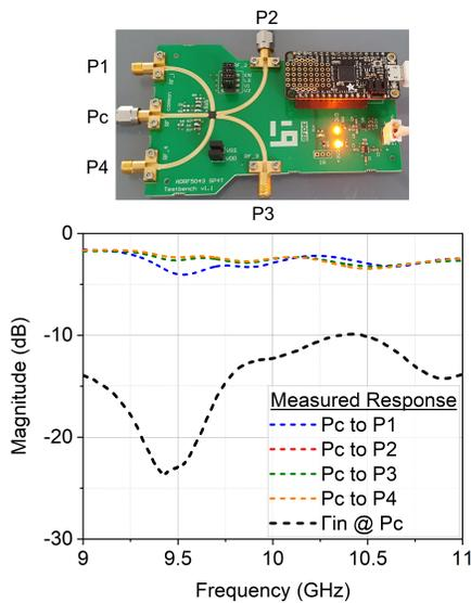
Fig. 9: Developed input-switching multiplexer module and the measured response
