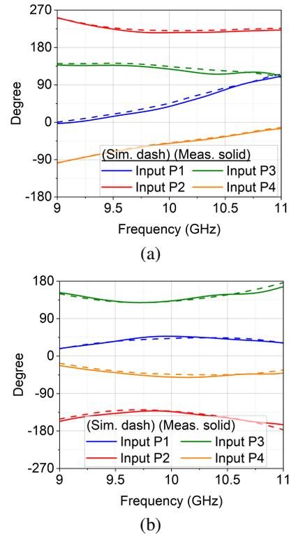
Fig. 5: Phase response between (a) Port 5 and 6, and between (b) Port 6 and 7 of the Butler matrix
