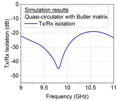
Fig. 14: Simulation results for the TRx isolation of the quasi-circulator connected to the Butler matrix
