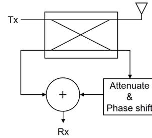
Fig. 10: Block diagram of the designed quasi-circulator
