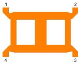
Fig. 1: Layout ( $14 \times 9 \text{ mm}^2$ ) of microstrip cross over
