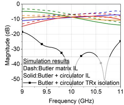
Fig. 15: Simulation results for Tx-to-antenna insertion loss and TRx isolation for the quasi-circulator integrated with Butler matrix through matching network
