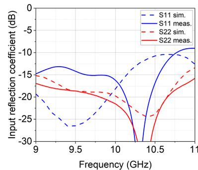
Fig. 6: Input return loss of the Butler matrix
