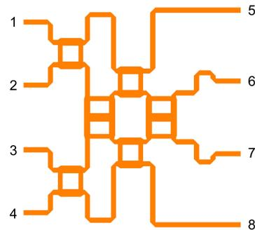
Fig. 3: Layout ( $53 \times 54 \text{ mm}^2$ ) of the Butler matrix
