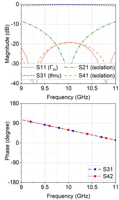
Fig. 2: Simulation results for microstrip cross over
