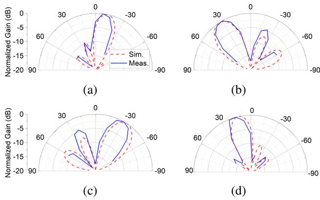
Fig. 8: Beam patterns generated by Butler matrix when excited by (a) Port 1, (b) Port 2, (c) Port 3 and (d) Port 4
