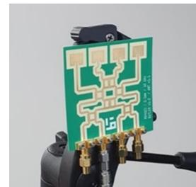
Fig. 7: Photograph of the developed Butler matrix
