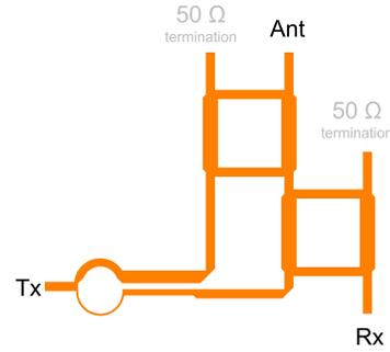
Fig. 11: Layout ( $16 \times 20 \text{ mm}^2$ ) of the quasi-circulator (Ant= Antenna)
