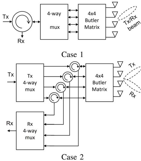
Fig. 13: Integration of Butler matrix with quasi-circulator (mux = multiplexer)
