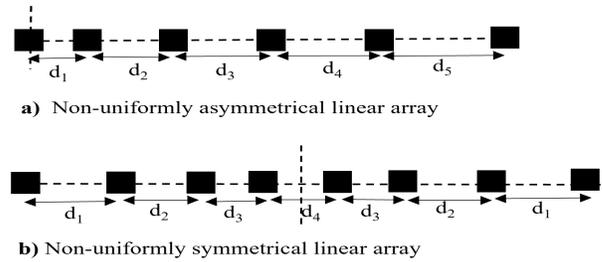
Fig. 3. Non-uniformly geometrical configurations
