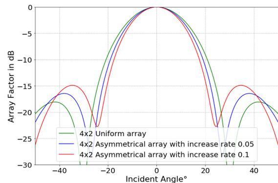
Fig. 7. Normalized Array factor patterns of 4x2 Uniform and Non-uniform Asymmetrical planar arrays
