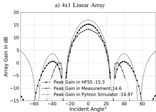
Fig. 6. Comparison of Gain Patterns
