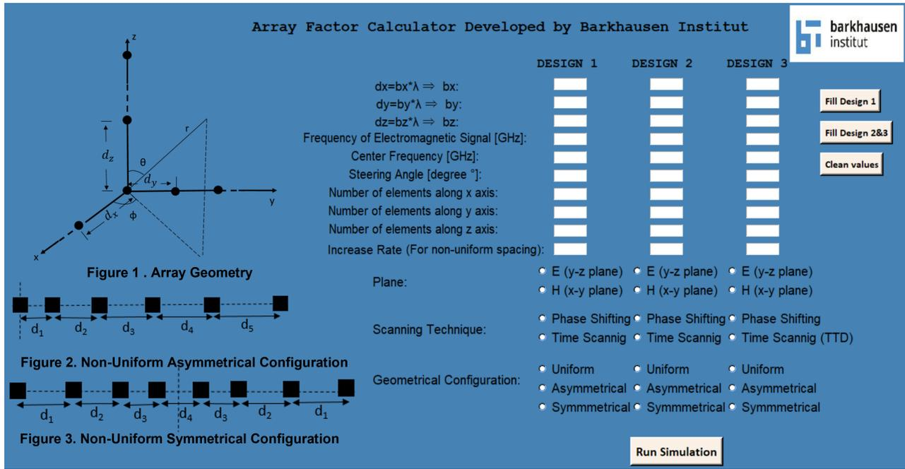
Fig. 2. GUI of Python-based Simulator's input window
