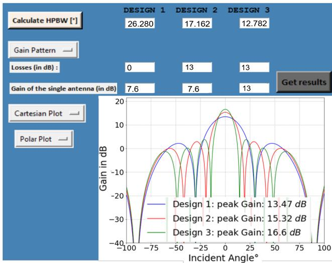
Fig. 4. GUI of Python-based Simulator's output window
