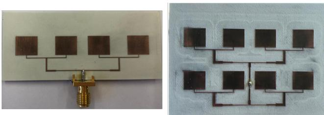
Fig. 5. Fabricated antenna arrays a) 4x1 Linear b) 4x2 Planar
