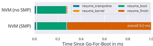
**Figure 3.** Latency breakdown for a resume-from-NVM operation on L4Re.
