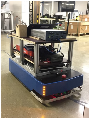
(a) Measurement hardware attached to a moving AGV.
