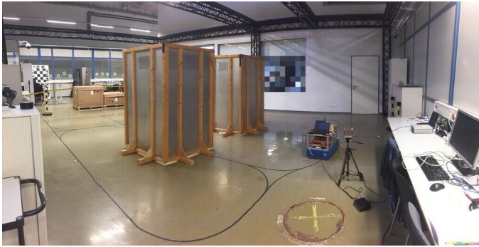
Fig. 3: The test site is modified by placing metal walls to create LOS and NLOS areas. The AGV moves around both obstacles. Figure 4a shows the corresponding map of this scenario.
