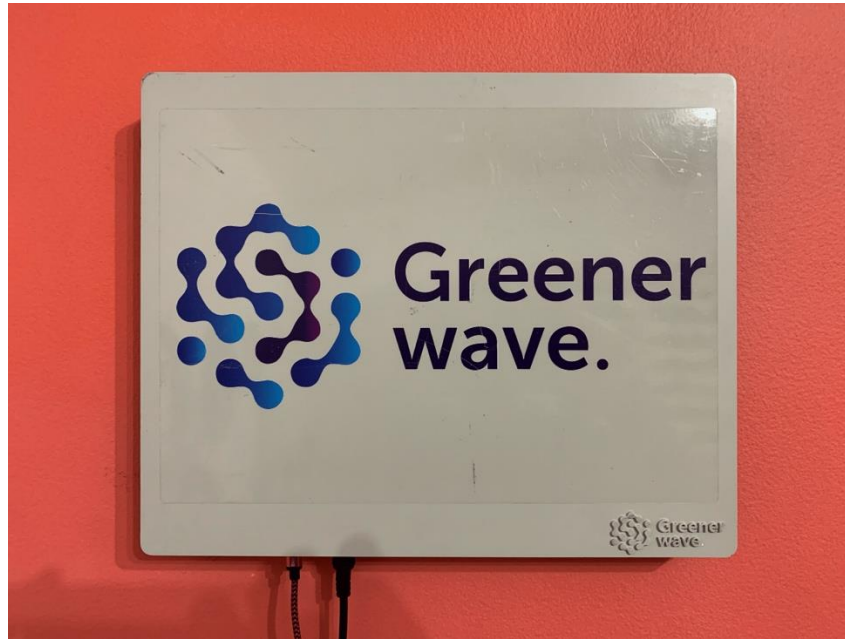
Figure 17: GW FR2 RIS mounted on a wall
