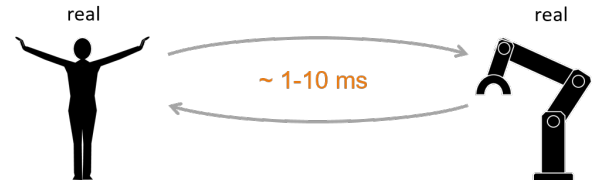
Fig. 2a: Direct remote control of a robot with strict ultra-reliable low-latency (URLLC) requirements
